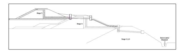
Figure 6.14: Cross-section of existing facility embankment
