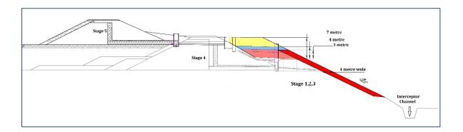
Figure 6.16: Cross section illustrating the extent of the proposed buttressing works
