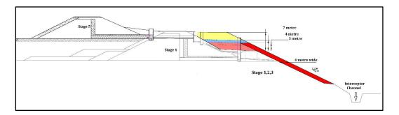
Figure 6.4: Cross section – facility embankment with buttress
